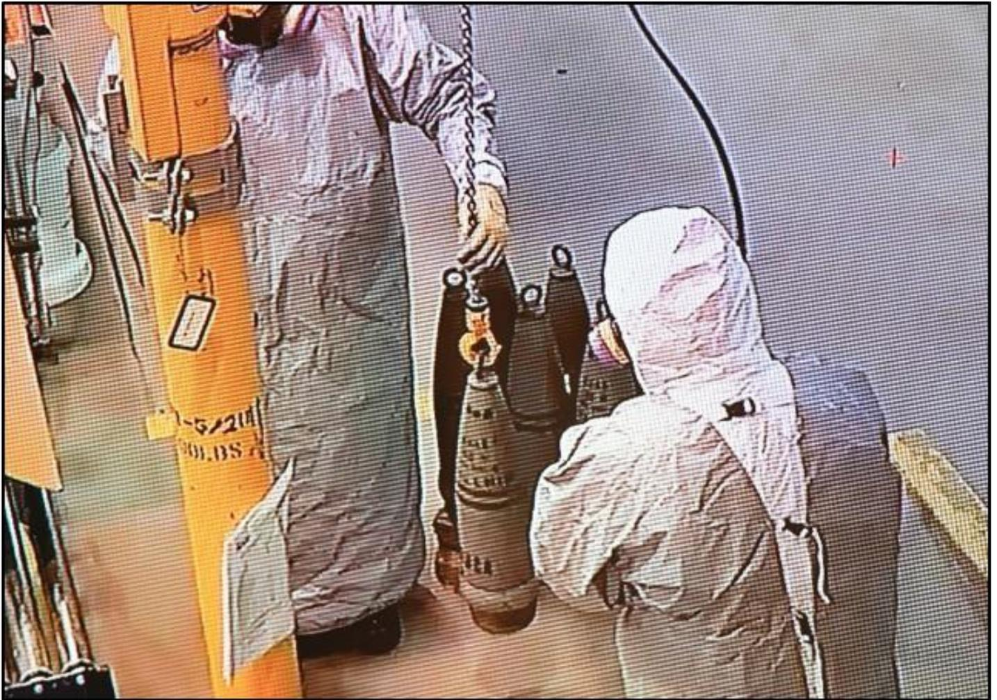
*Photo caption: Workers use a crane to lift the first 155mm projectile containing mustard agent to begin the destruction process in the Static Detonation Chamber at the Blue Grass Chemical Agent-Destruction Pilot Plant June 7, 2019. (Photograph from closed circuit television)*
