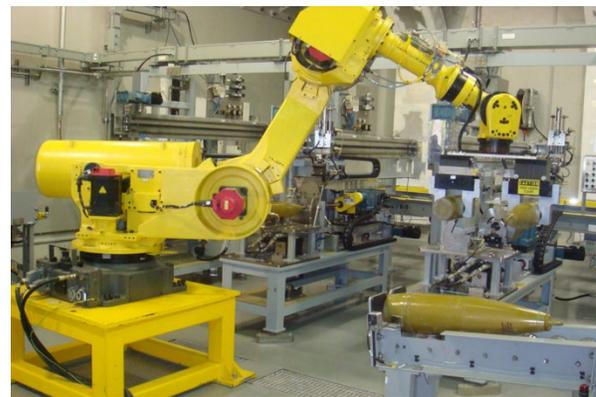
*The Projectile/Mortar Disassembly system's robotic technology ensures the safe and efficient removal of the explosive components from the chemical munitions.*
