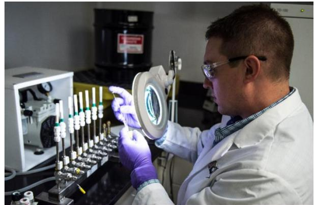
*A Blue Grass Chemical Agent-Destruction Pilot Plant Laboratory staff member analyzes Depot Area Air Monitoring System, or DAAMS, tubes. The perimeter monitoring stations, using DAAMS, will provide historical monitoring to augment near real-time monitoring at the plant.*
