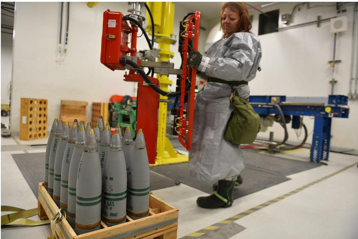
An ordnance technician uses a lift assist to transfer a 105mm projectile onto a pallet.
