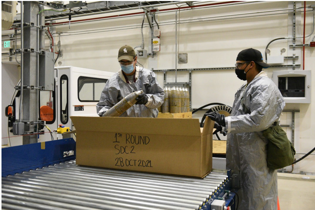
A Pueblo Chemical Agent-Destruction Pilot Plant ordnance technician places an inert 4.2-inch mortar round into a feed box placed on a processing line during Static Detonation Chamber trial burn testing on Oct. 28, 2021.
