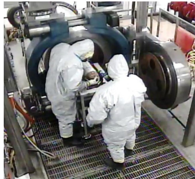
March 18, 2015 – The first mustard agent from the Pueblo stockpile to be destroyed is loaded into the EDS.
