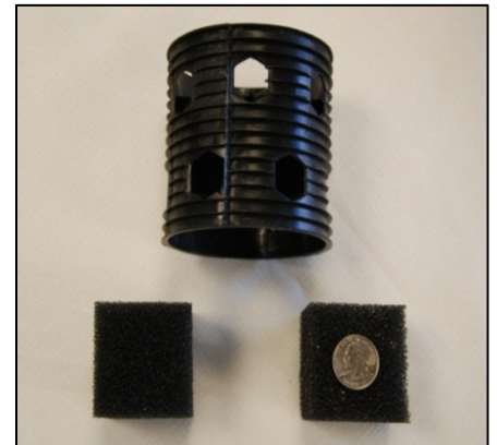
Sandwiched between the various immobilized cells in the PCAPP bioreactors, is an assortment of polyurethane foam cubes, in which the wastewater eating microbes will reside.
