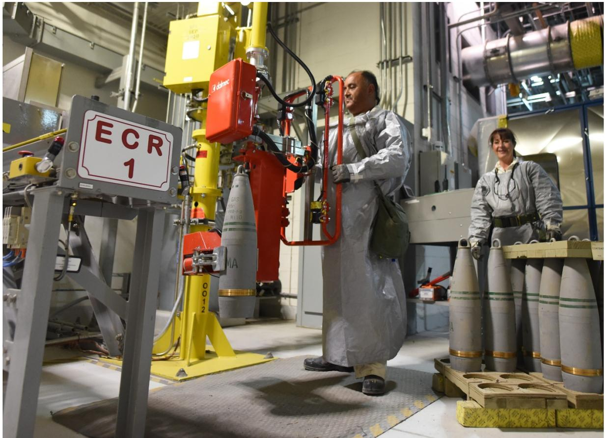
A Pueblo Chemical Agent-Destruction Pilot Plant ordnance technician uses a lift assist to transfer a 155mm projectile onto a conveyor belt prior to destruction in fall 2019. Conveyors transport munitions into Explosive Containment Rooms where energetics are removed from projectiles before the chemical agent contained within is drained and neutralized.
