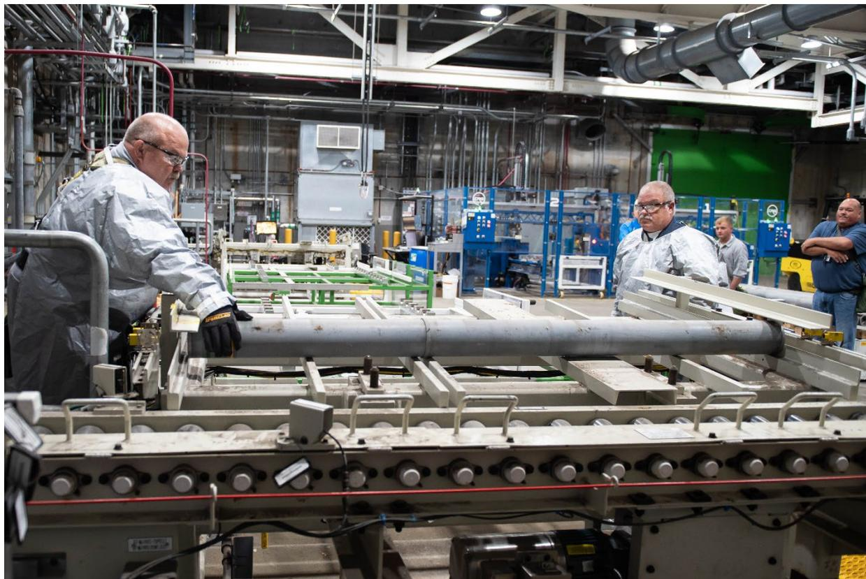
*Photo caption: Blue Grass Chemical Agent-Destruction Pilot Plant operators place the first M55 rocket containing GB nerve agent on a conveyor to begin the destruction process July 6, 2022. The GB nerve agent M55 rockets are the last type of chemical weapons to be destroyed in Kentucky. (U.S. Army photo)*
