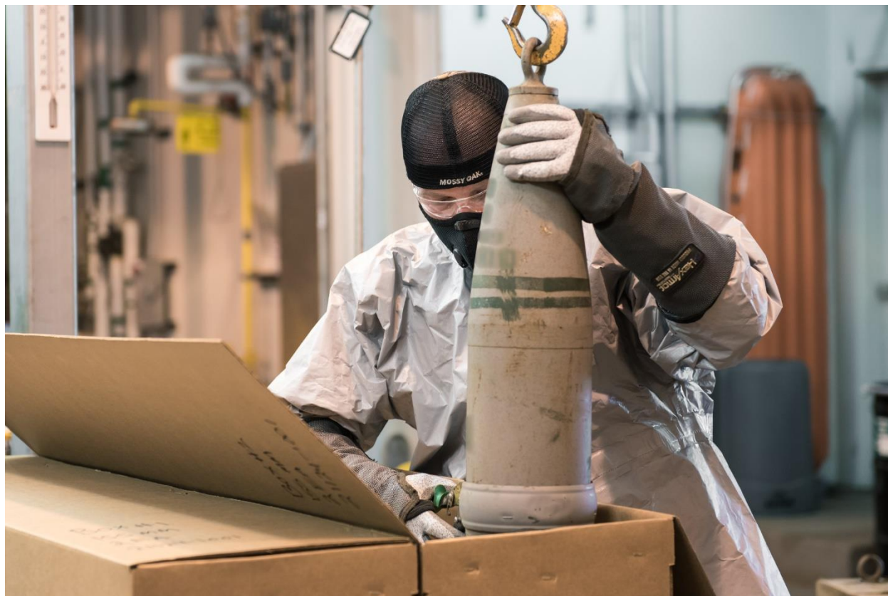
Photo caption: A munitions handler places a 155mm projectile containing mustard agent into a box to begin the destruction process in the Static Detonation Chamber at the Blue Grass Chemical Agent-Destruction Pilot Plant. (A portion of this photograph has been blurred in accordance with Department of Defense guidelines.)
