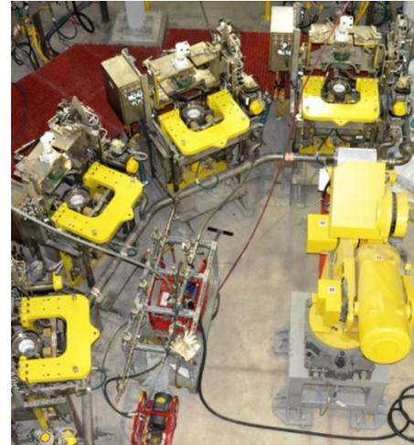
*Projectiles and mortars entering the Agent Processing Building will first visit a station called the Munitions Washout System, which consists of two Cavity Access Machine arrays that have four lines each.*
