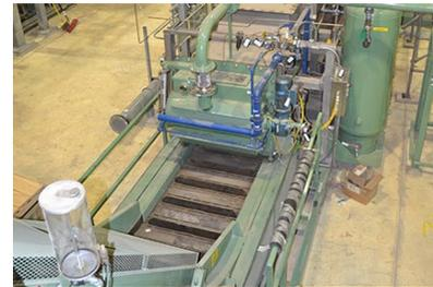
*Munitions Treatment Units heat decontaminated munition shells to 1000 degrees Fahrenheit.*
