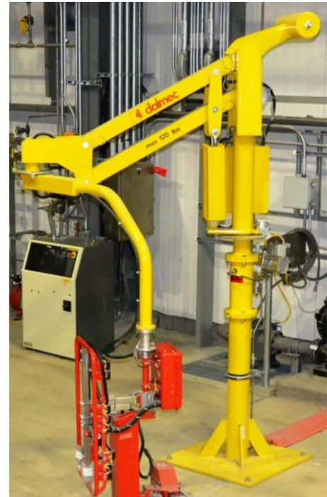
*Munitions Handling Lift Assist devices will be used in both the Enhanced Reconfiguration and Agent Processing Buildings to safely transfer munitions between process equipment pallets.*
