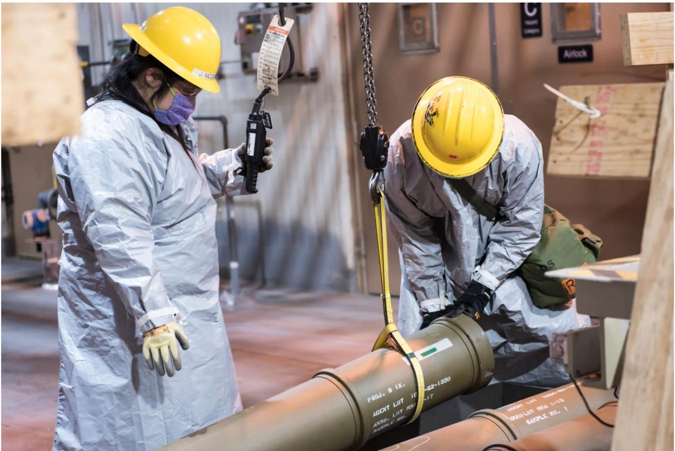
*Photo caption: Two operators work together to place one of the last overpacked 8-inch projectiles containing nerve agent into a tray to begin the destruction process at the Blue Grass Chemical Agent-Destruction Pilot Plant May 9. The last GB 8-inch projectile was destroyed May 11, marking the complete destruction of an entire type of chemical weapon.*
