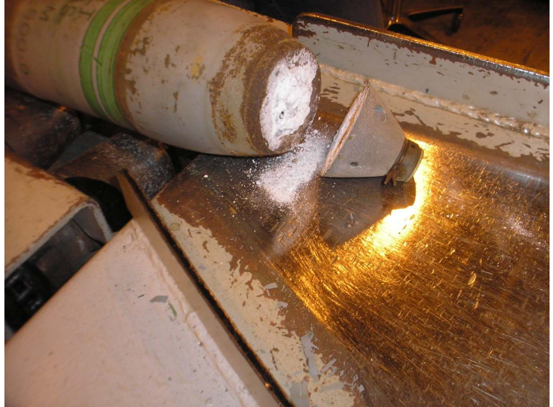
Fuze falls off a 4.2" mortar during processing at ANCDF
