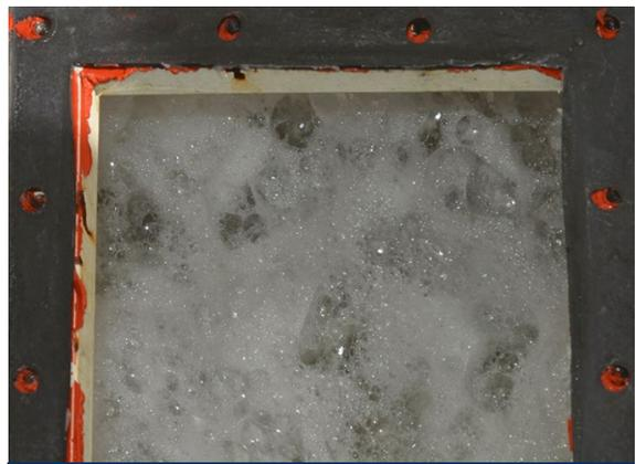
*Thriving microbes inside the bioreactors treat hydrolysate, the wastewater product resulting from the chemical agent neutralization process.*
