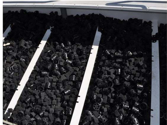
*Sandwiched between the various immobilized cells in the PCAPP bioreactors is an assortment of polyurethane foam cubes, in which the wastewater-eating microbes reside.*
