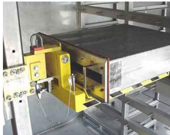
*Lifting devices, such as the one pictured here will aid operations should replacement of carbon filters inside the units in the Agent Filtration Area become necessary to maintain optimum performance during chemical demilitarization*
